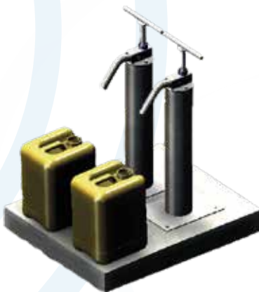
Multiple equipment on the same 4" and greater borehole
