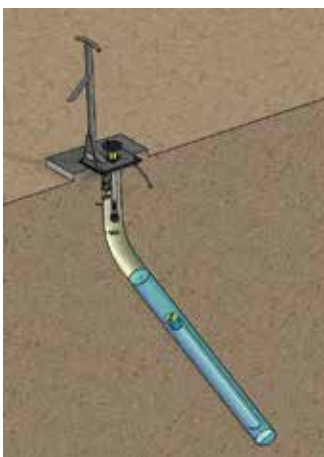
Installation possible in a non-vertical borehole
