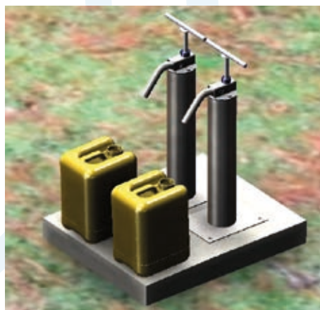
Multiple equipment on the same 4" and greater borehole
