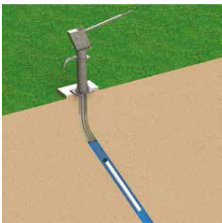
Installation possible in a non-vertical borehole
